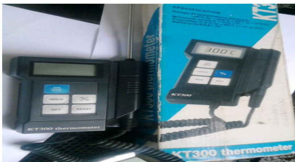
Fig 3.1 Digital thermometer KT300 used in obtaining temperature reading from the different transects in the Douala urban space
