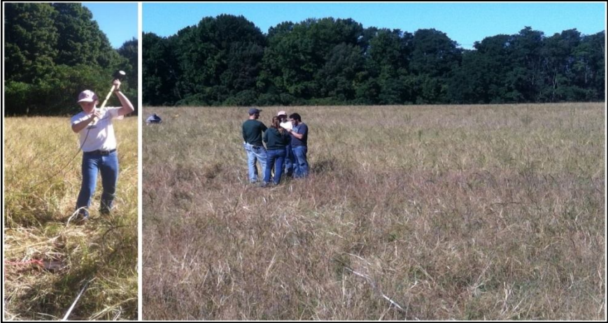
Figure 4: Field survey. Left) Sledge hammer being used as a seismic source, Right) Field crew setting up seismic surveying equipment.
