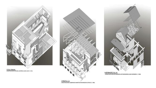
Exploded axonometric views of traditional Puerto Rican architecture, showing construction materials and assembly procedures. Drawn using strictly AutoCAD.
