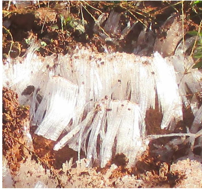
Figure 4 – Needle ice at a construction site in Boiling Springs, South Carolina, December 20, 2015. Little soil was lifted by the needles indicating water was near the surface of the soil and freezing started near the top of the soil. The base of the needles is separated from the soil. This is an illustration of clear needles in abnormally wet conditions.
