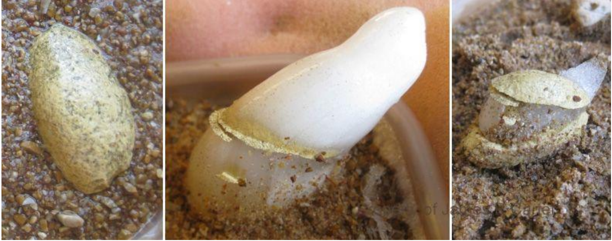
Figure 14 – Three views of a dome-shaped pebble 3-cm long that had been a regular producer of segregated ice. The center view shows that a large column of ice grew from the top of the pebble and then the pebble split horizontally and subsequently ice grew from the base of the split. The view on the right shows the split pebble after most of the ice on top melted. Photos June 12, 2012
